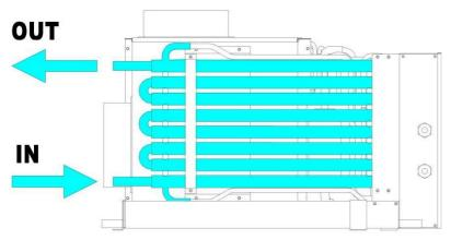
Connect the self-contained heat exchanger unit in the following manner:
