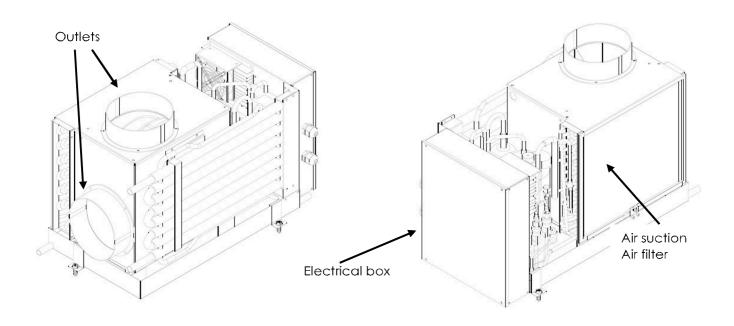
**IMPORTANT!** Both outlet fittings can be ducted allowing the highest air flow rate, however in case of restricted space for installation, only one outlet can be ducted while the other shall be closed. For Compact i27 VSD at least two outlets must be used.
