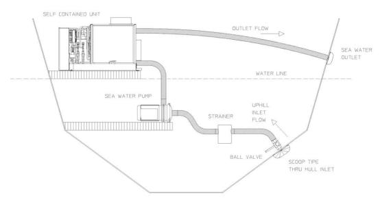
The minimum nominal diameter of the connecting pipes should be 1/2".
