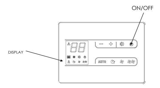
The room thermostat has to be connected with the PCB through the 5 m cable (supplied with the unit).
