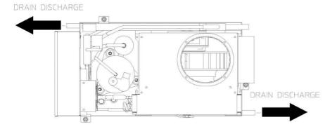
**NOTE:** The direct discharge at side is not recommended because of sucking bad smells from the outside caused by the exhaust gas of its own or other engines.
