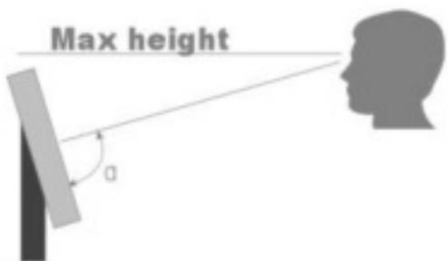
Viewing angle is an theoretical value measured with standard colors and contrast. In real life the monitor should be installed with angle:  $120 < \alpha < 90$ . This means that viewing from bottom side should be avoided. For viewing convenience install the monitor below eye-level (max height).
