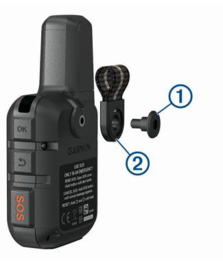
2 Secure the spine mount adapter 1 over the back of the device using the long screw 2 included with the device.
