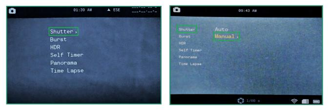
4. To set the shutter settings manually, toggle down to Manual and right to the shutter speeds.
