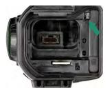
3. Press the tab on the left side of the battery and slide the battery out. Slide the Viewfinder back into its slot.
