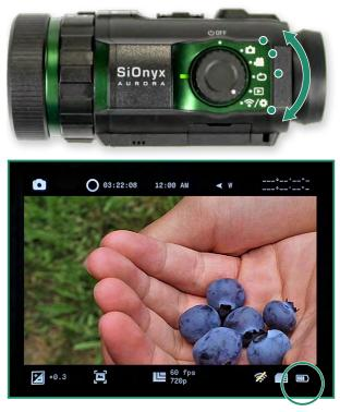
The battery gauge icon is on the bottom right of the screen.
