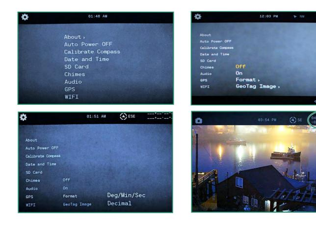
**Note:** GPS only works when you're outside and requires 1-2 minutes for the camera to receive an initial location. GPS consumes power and should be turned off to extend battery life when not in use.
