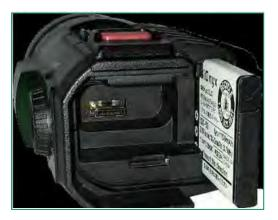
4. Slide the battery into the battery slot.
