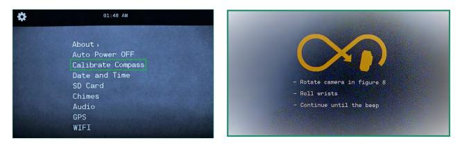
If the compass fails to calibrate, you'll hear a boing sound and see a message that says: "Retry compass calibration."
