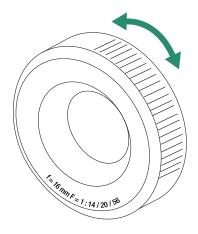
**Note:** To assist in focusing, estimate the distance where the action in your scene will occur and set that distance in meters on the focus scale. You can also turn on Focus Peak under the Overlay menu.
