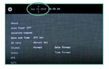
6. Select the Date Format at the top of the screen. Select an option and press SET. See "Section 4.4.2 Format".
