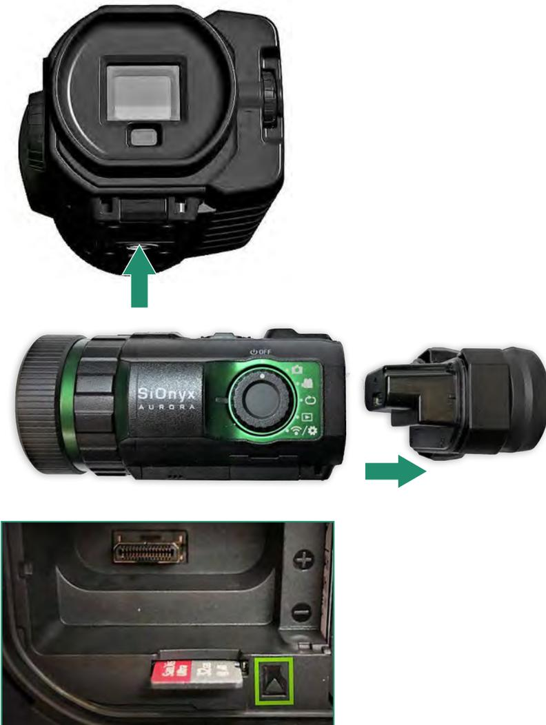
**Note:** Don't force the SD card into the slot or the data may be damaged.
