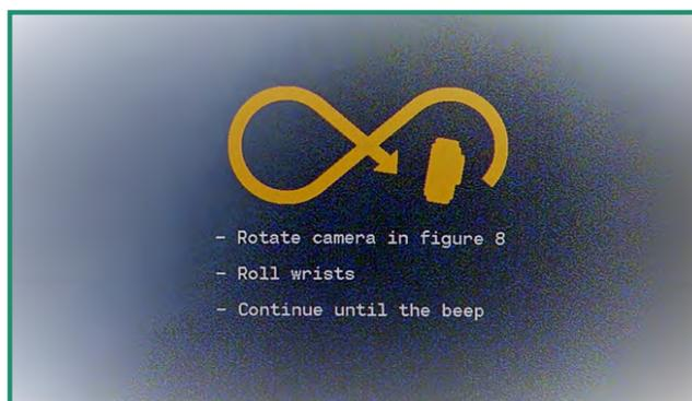
*If the compass fails to calibrate, you'll hear a boing sound and see a message that says: "Retry compass calibration."*
