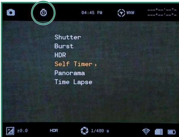
When you press the Shutter button chimes will sound to count down the delay, followed by a click when the picture is taken.
