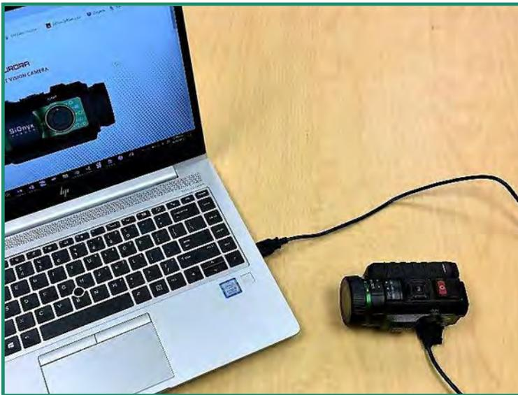
A green light appears and blinks slowly during the charging process. When the battery is fully charged, the light will turn off.
