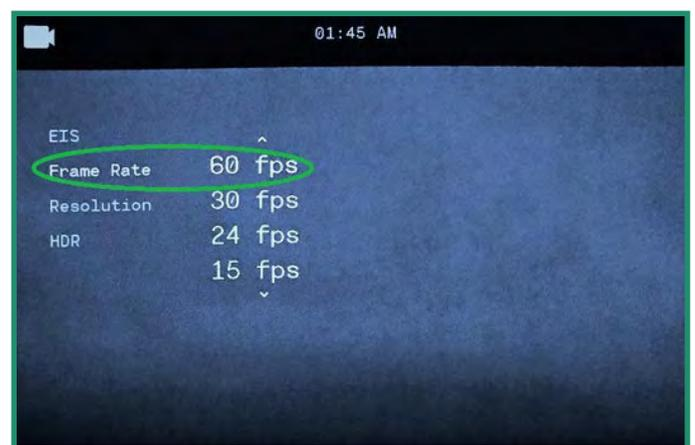
**Note:** 60 fps will generally produce a smooth looking video. You can set the frame rate from 60 fps to Slo Mo. The Frame Rate will be displayed at the bottom of the Viewfinder. For best results when using the Day setting on the Scene Ring, select 60 fps. With the Twilight or Night setting, select 30 fps or slower.
