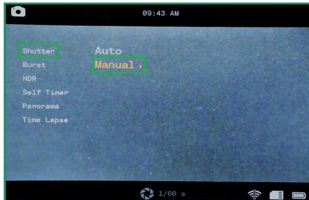
4. To set the shutter settings manually, toggle down to Manual and right to the shutter speeds.
