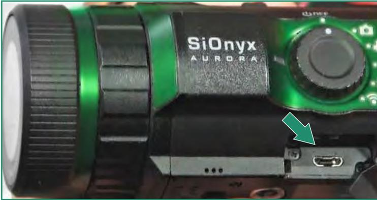
6. Connect the camera to a powered-on PC using the supplied Micro USB cable.
