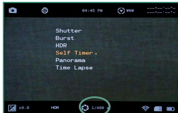
5. Toggle up and down to scroll through the shutter speed settings.
