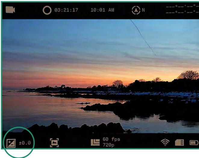
The Exposure Compensation/Gain setting is located on the bottom left of the Viewfinder menu.
