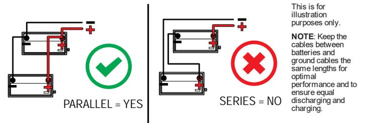
**How to connect batteries in parallel:**
