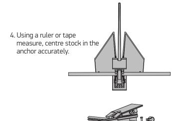
5. Slide clips onto stock and fix through the flukes and tighten nuts and bolts.
