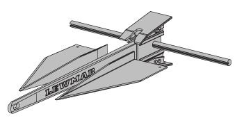
3. Slide flukes into the groves both sides of the crown.
