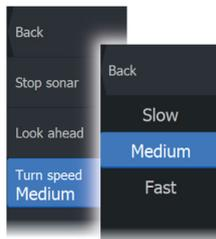
Use this option to set the rotation speed of the transducer. Select one of the following turn speeds:
