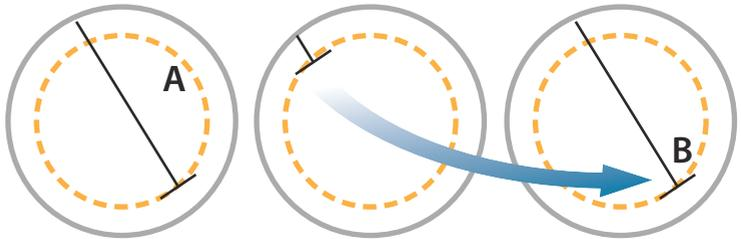
When true motion is selected, the true motion reset option is available from the menu. This allows for manually resetting the radar image and vessel symbol to its starting position.
