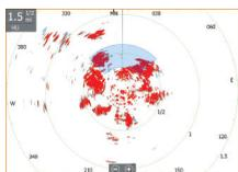
A guard zone is an area (either circular or a sector) that you can define on the radar image. When activated, an alarm alerts you when a radar target enters or exits the zone.
