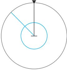
The electronic bearing line (EBL) and variable range marker (VRM) allows quick measurements of range and bearing to vessels and landmasses within radar range. Two different EBL/VRMs can be placed on the radar image.
