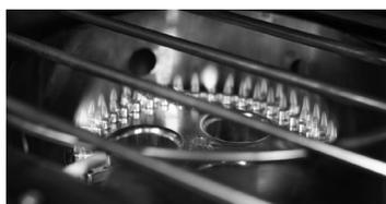
Normal flame should be all blue and look like its touching the burner at the bottom, with a minimal amount of yellow/orange.
