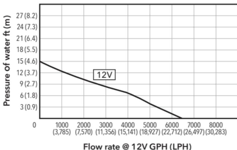
All pumps are tested at nominal voltage with fresh water at ambient temperature with no ports attached.
