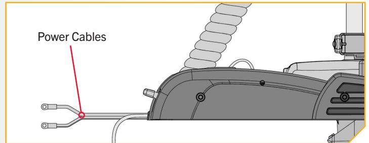
**NOTICE:** The PowerDrive has no power switch. When the Power Cables are connected to a battery, the PowerDrive is "on". When the Power Cables are disconnected from the battery, the PowerDrive is "off". If the Power Cables are connected to a breaker, the PowerDrive is "on" when the breaker is "on" and "off" when the breaker is "off".
