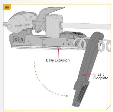
Replace the four sideplate screws using a #3 or #2 Phillips screwdriver. Two of these screws will be located on each side of the mount.
