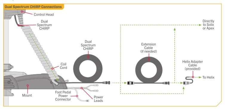
All Dual Spectrum CHIRP PowerDrive motors are equipped with an internal bonding wire. Incorrect rigging will cause sonar interference and can damage your trolling motor, electronics, and other boat accessories. To minimize trolling motor interference, ensure that the fish finder and trolling motor are powered by separate batteries. Please refer to the "Battery & Wiring Installation" and "Motor Wiring Diagram" sections of this manual for correct rigging instructions.
