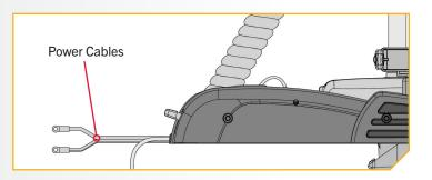
**NOTICE:** The PowerDrive has no power switch. When the Power Cables are connected to a battery, the PowerDrive is "on". When the Power Cables are disconnected from the battery, the PowerDrive is "off". If the Power Cables are connected to a breaker, the PowerDrive is "on" when the breaker is "on" and "off" when the breaker is "off".
