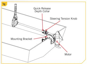
**NOTICE:** This motor weighs approximately 30 lbs. We recommend having a second person help with the installation.
