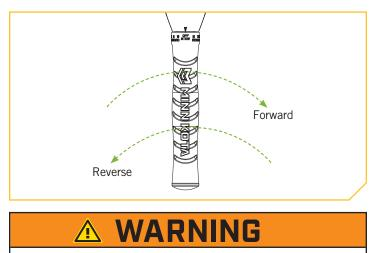
Be alert for unexpected boat movement when operating the Traxxis. The boat may encounter sharp turns and jolts if the steering is changed sharply or if broad changes in speed are made while operating. Maintain balance and observe safe motor operation.
