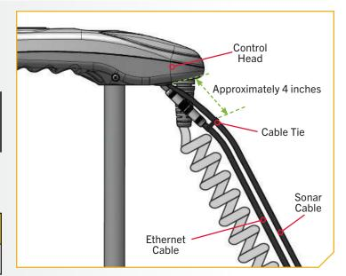
Follow the Cables from the Control Head to the Mount and place additional Cable Ties every 4 inches around the Cables after the first Cable Tie. The number of Cable Ties needed will vary depending on the length of your trolling motor Shaft.
