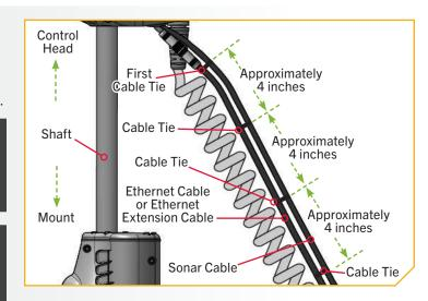
Continue placing Cable Ties around the Accessory Cables until there are two Cable Ties in place past the end of where the Coil Cord enters the Mount.
