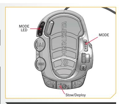
**NOTICE:** The deploy sequence can be stopped at any time by pressing the Stow/Deploy button. The stow sequence can be stopped at any time by pressing either Trim buttons or the Stow/Deploy button.
