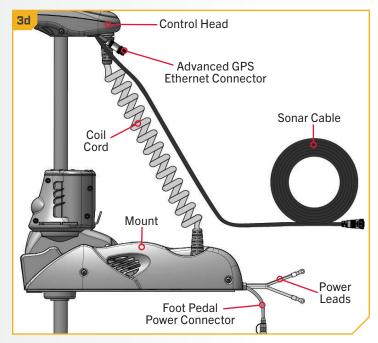
**NOTICE:** CRITICAL CABLE ROUTING. On motors with a 60" shaft, accessory cables must exit the Coil Cord leaving three or more open coils between where the cables exit and the motor base, as assembled by the factory. Routing the cables in any other manner will not allow the motor to stow properly. Please see the "Securing Accessory Cables" section of this document for details.
