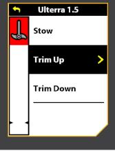
the bottom of the mount to the center of the lower unit. A lower trim limit is set approximately 1.5" from the bottom of the control head to the trim housing. A prop lockout region, defined as 14" from the bottom of the mount to the center of the lower unit, is used to eliminate the possibility of the motor contacting the boat hull. All functions, with the exception of manual steer and track record, are canceled upon trimming into this region.
