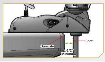
**NOTICE:** Failure to allow 1-1/2" of clearance for the Shaft when mounting may cause failures when the motor stows and deploys. Follow recommended mounting considerations to avoid obstructions when operating the motor.
