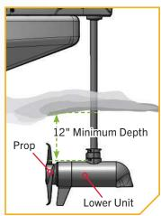
**NOTICE:** To avoid churning or agitation of surface water, ensure that the top of the motor is submerged at least 12" below the surface of the water.
