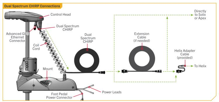
All Dual Spectrum CHIRP Ulterra motors are equipped with an internal bonding wire. Incorrect rigging will cause sonar interference and can damage your trolling motor, electronics, and other boat accessories. To minimize trolling motor interference, ensure that the fish finder and trolling motor are powered by separate batteries. Please refer to the "Battery & Wiring Installation" and "Motor Wiring Diagram" sections of this manual for correct rigging instructions.
