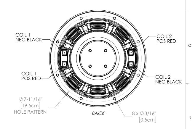
Item NumberImpedance48CWRT822OHM DVC48CWRT844OHM DVC
