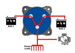
4 Position Switch Controls Which Battery (or both) Supplies a Single Output
