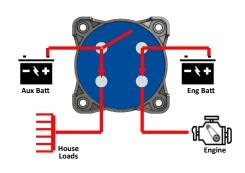
3 Position ON/OFF Switch Controls Two Circuits, With the Option To Combine Batteries
