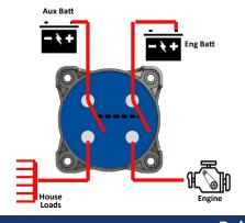
2 Position - ON/OFF Switch Controls Two Independent Circuits
