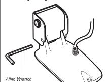
**Tightening the Pivot Screw**
