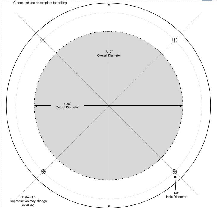
**Installation:** Find a suitable location making sure there is clearance for the installed depth. Use a hole saw or other suitable device to make a cutout.
