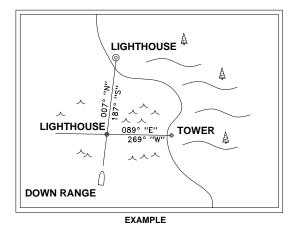
**Step Three.** Simply repeat steps 1 & 2, except this time, using an East/West course and the <u>fore/aft compensator (slot is facing aft).</u>
