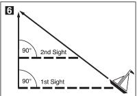
by the time equals both your distance offshore (A) and the distance run (B). Tip: Another method to determine distance offshore is to take two sightings off the same object exactly 60 minutes apart and plot the two lines of position. Open a pair of dividers to match your distance traveled in 60 minutes. Draw your actual travel line of position (A) parallel to the compass course you are steering at the point where the angle is the same width as your distance traveled (figure 5).
