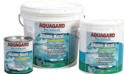
Alumi-Koat is an acrylic copolymer, cuprous oxide pigmented coating formulated especially to prevent barnacles, algae, slime and other fouling organisms on vessels immersed in salt, brackish and fresh water. Non-toxic fumes, soap and water clean-up. Superior adhesion to aluminum, no barrier coat required. Controlled leach out. Paint can be applied over existing bottom paints that are clean, free of any debris and dry. U.S. EPA approved. Plastic container increases shelf life.
