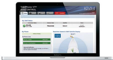
Start your web browser and enter **http://minivsat.kvh**. If this web address doesn't work on your platform/browser, enter the ICM's IP address (you can find this address on the LCD: go to Settings > Network Settings > IP Assignments).
