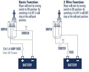
Standard Motor (Customer Supplies Wires)
