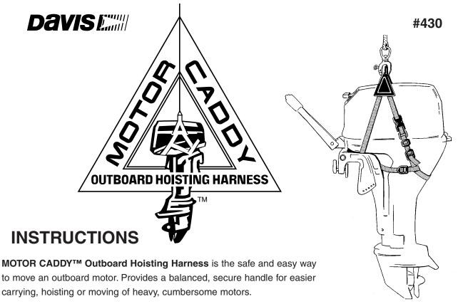
Fits 2-stroke and 4-stroke outboards up to 15 h.p. Motor Caddy is sized to quickly attach onto most outboards from 2–15 horsepower. (Not recommended for air cooled motors).
