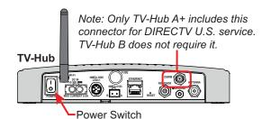
At the rear panel of the TV-Hub, set the power switch to the On position. The TV-Hub supplies power to the antenna. Wait a few minutes for system startup.
