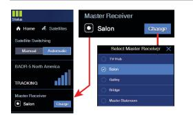
If your system is set up for automatic satellite switching with multiple receivers, you can select the master receiver on the Home page of the web interface. The master receiver controls satellite selection.
