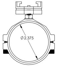
Bigg Rigg Outrigger Main Base Tube (Below 1st Spreader)
