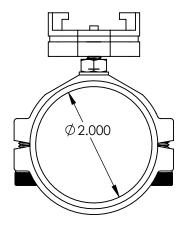
**Tournament Outrigger** Main Base Tube (Below 1st Spreader)
