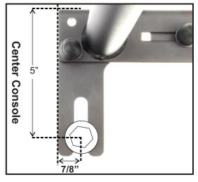
If you are using Orientation B from Step 1, the distance between the seat bolts and center console must be at least 5".
