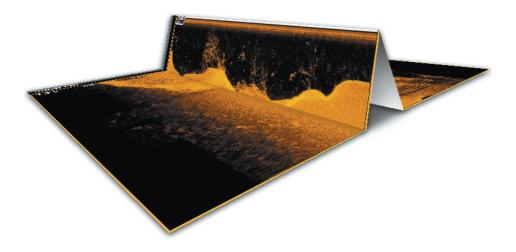
To visualize how Side Imaging works, the Side Imaging View illustration can be folded down the middle and then folded again at the lowest point of the water column. The raised area reveals the water column with its relative depth of the water under the boat. In the Side Imaging View, variations in the width of the water column show variations in the distance to the bottom as the boat passes over.
