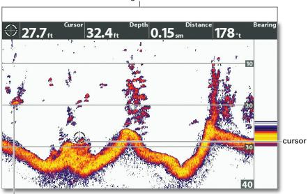
**Sensitivity** on the Sonar X-Press Menu can be adjusted to display more or less sonar returns on the screen.
