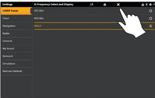
Press the EXIT key to close a menu or go back one level. Press and hold the EXIT key to close all menus.
