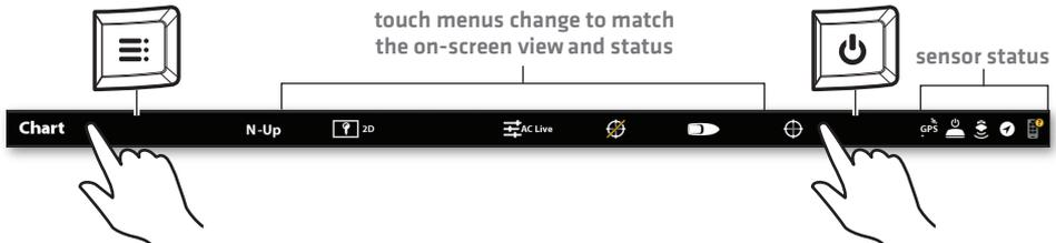
Tap the view name or press the MENU key to open the X-Press Menu for the on-screen view.
