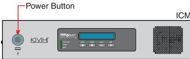
Press the power button on the ICM then wait 5 minutes for system startup. When the ICM indicates "Online," you can make a voice call or access the Internet using any device connected to the network.
