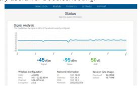
The top graph shows your Hotspot's signal over time. Dropouts usually indicate an issue at the Hotspot itself, or some object blocking your line of site to the antenna.
