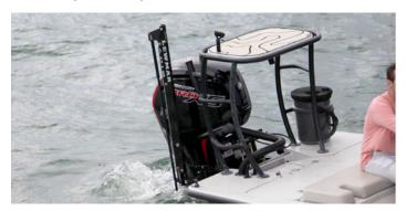
With no hydraulic pump and hoses to worry about the shallow water anchor can be installed quickly and takes up less space.
