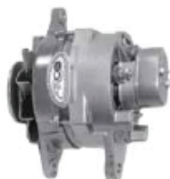
Brush Cover Installed
