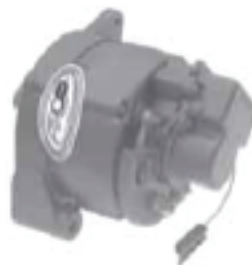
Brush Cover Installed
