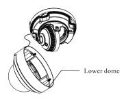
(§) Connect the cables, mount the rubber plug to the gap of the mounting base and fasten the camera onto the junction box.
