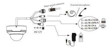
\* It is recommended to install the water-proof connector for outdoor installations.
