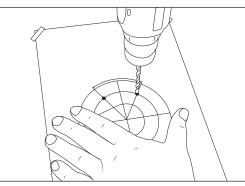
Clean the mounting surface and tape the drilling template in position so that it
