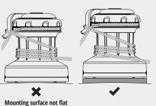
Ensure the Drive gear is aligned to the line entry as per the orientation on
